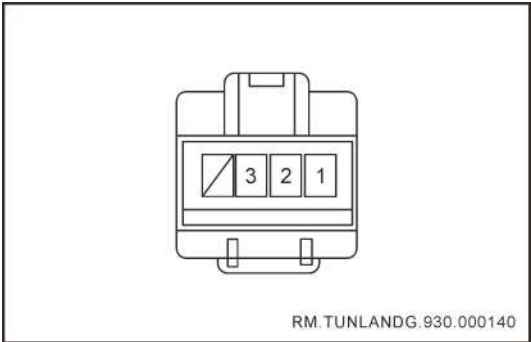
3A04FW Hu Lian F003 into Rear overhead light assembly
